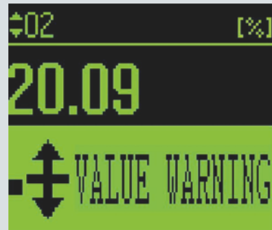
Local user interface (LUI) of SITRANS SL in the detector unit (display of measured value)
